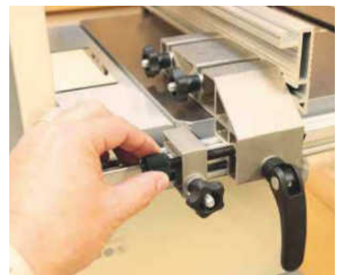
The fence locks with a cam lever and has a fine adjuster built in
